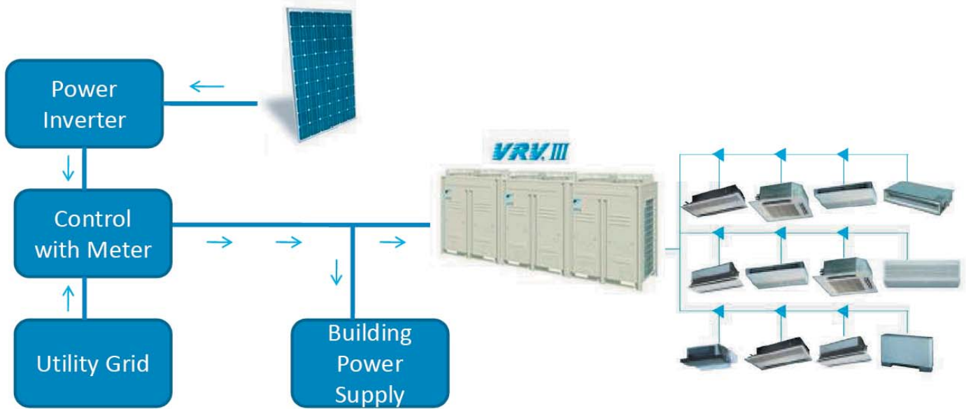
Figure 2: System Configuration of VRV with Photovoltaic.
